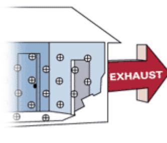
The [LionKing](#) Power Blower's unique shroud design creates the "cone of air" that is essential for PPV to work. In addition, the multiple blades of the AirFlex Impeller create the pressure required to get the air moving.
